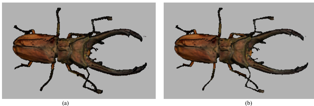
Fig. 15 The results of rendering "Beetle" range data. (a) without culling. (b) with culling.
