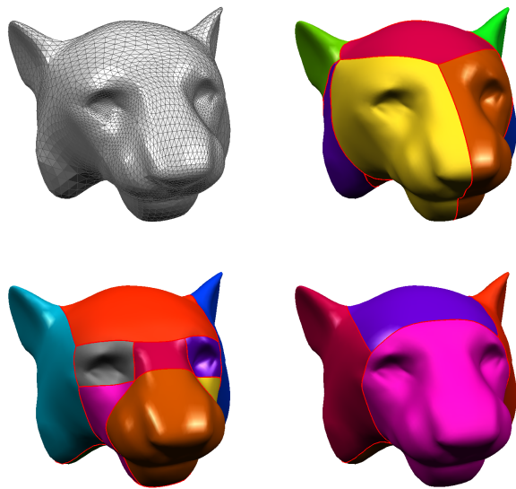
Figure 4: Various mesh decomposition results for “tiger’s head” mesh (4,034 vertices). The number of parametric curves for decomposition is 22, 26, and 12 respectively (from left to right).
