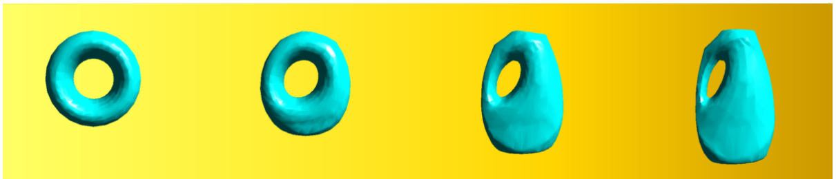
Figure 15: Result of metamorphosis from the “torus” model to the body of the “bottle” model as a simple example of the non-zero genus ( g = 1 ) objects. We have defined 17 CVPs. and a partition control mesh (17 vertices, 35 edges, and 18 faces) for the control of surface correspondence.
